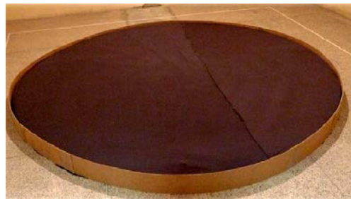
Fig. 2. The QRD covered with fabric used in the scattering coefficient measurement.
