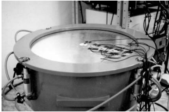
Fig. 1. Circular plate with sensors and actuators.
