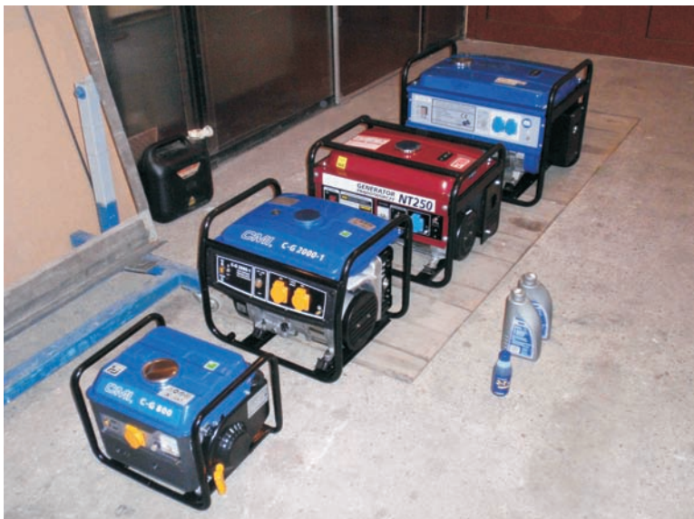
Fig. 3. Gasoline engine-generators prepared for acoustic measurements.
