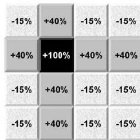
Fig. 8. Image of crosstalks in the model of a passive matrix, after activation of a transducer in the second column from the left and third row looking from the bottom.
