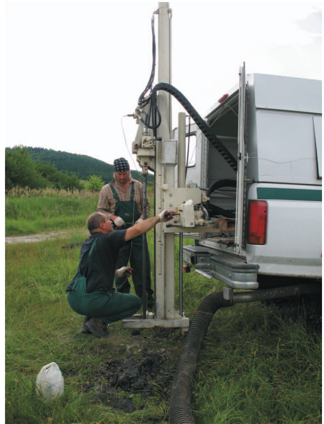
Fig. 14. Penetrometer-based resistivity profiling made by workers of Geofizyka Toruń Company. Photo by W. J. Mościcki
