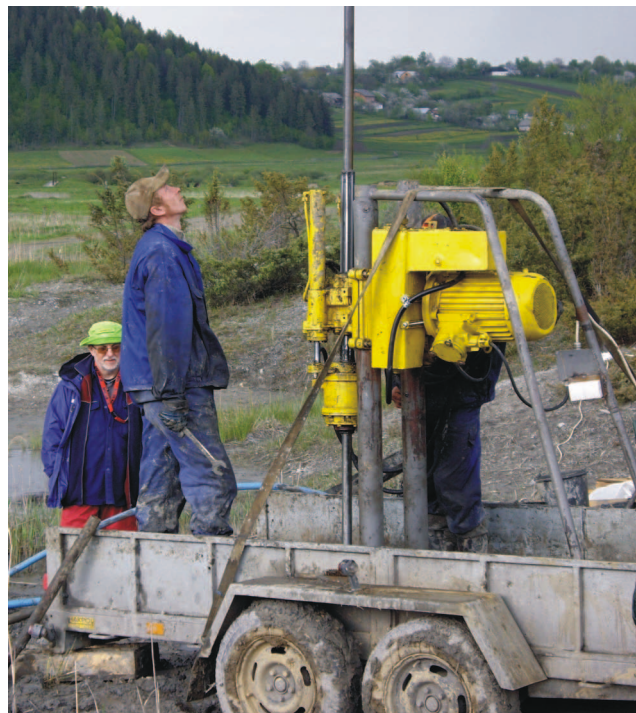
Fig. 11. The geological drillings by means of MDR-06 drilling probe with plexiglas inner tube (5 cm diameter). Photo by R. Stachowicz-Rybka
