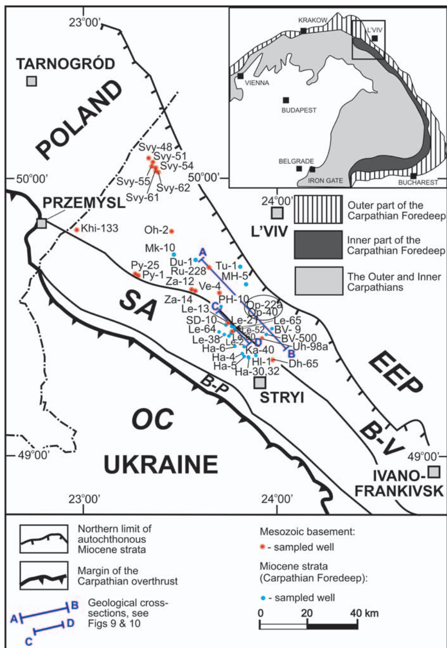
Fig. 1. Sketch map showing the major tectonic units of the Ukrainian Carpathian region and locations of gas sampling sites. EEP – East European Platform, B-V – Bilche-Volytsia Unit (outer part of the Carpathian Foredeep), SA – Sambir (Stebnik) Unit, B-P – Boryslav-Pokuttya Unit, OC – Outer (Flysch) Carpathians
