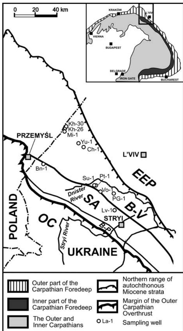
Fig. 1. Sketch map of major tectonic units of the NE part of the Ukrainian Carpathian region with the location of gas sampling sites. EEP – East European Platform, B-V – Bilche-Volytsia Unit (outer part of the Ukrainian Carpathian Foredeep). SA – Sambir (Stebnik) Unit, B-P – Boryslav-Pokuttya Unit, OC – Outer (Flysch) Carpathians
