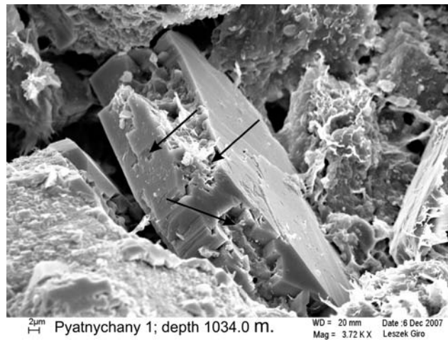
Fig. 10. Dissolution traces (arrows) of dolomite. SEM image; Pyatnychany 1 well; depth 1,034.0 m
