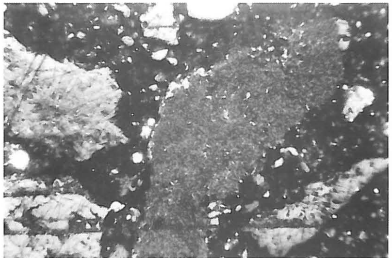
Fig. 3. Sample after one week of leaching — effect of the sulphur bacteria
