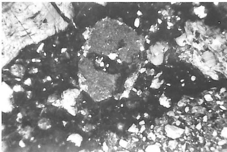
Fig. 9. Effect of bacteria — isolated residues of pyrite in edges
