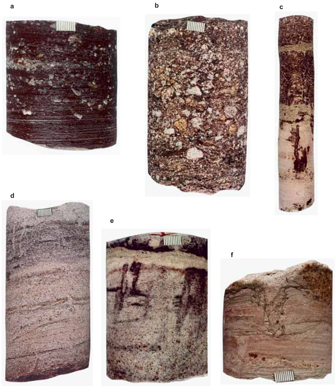
Fig. 29. Scale marked in millimeters; a — facies Mm — massive mudstone with scattered fine pebbles; Malbork IG 1 borehole, depth 3657.7 m; b — facies Cm — grain-supported massive conglomerate; transitional complex — continental-marine deposits; Olsztyn IG 2 borehole, depth 2709.1 m; c — at the bottom: facies Sh (subfacies ShS) — horizontally laminated fine-grained sandstone with admixture of fine pebbles; note vertical burrows; above: facies Sm (subfacies SmP) — massive medium- and coarse-grained pebbly sandstone; transitional complex — continental-marine deposits; Olsztyn IG 2 borehole, depth 2706.3 m; d — facies Sc (subfacies ScS) and Sh (subfacies ShS): large-scale cross bedded medium- and coarse-grained sandstone, passing upwards into horizontally bedded sandstone with vertical bioturbation structures; transitional complex — continental-marine deposits; Malbork IG 1 borehole, depth 3637.7 m; e — facies Sm (subfacies SmS) — massive medium- and coarse-grained sandstone with vertical bioturbation structures; transitional complex — continental-marine deposits; Malbork IG 1 borehole, depth 3640.4 m; f — facies Sh (subfacies ShS) — horizontally laminated fine-grained sandstone; a vertical burrow filled with very coarse-grained sandstone (subfacies SmS); transitional complex — continental-marine deposits; Olsztyn IG 2 borehole, depth 2703.6 m
