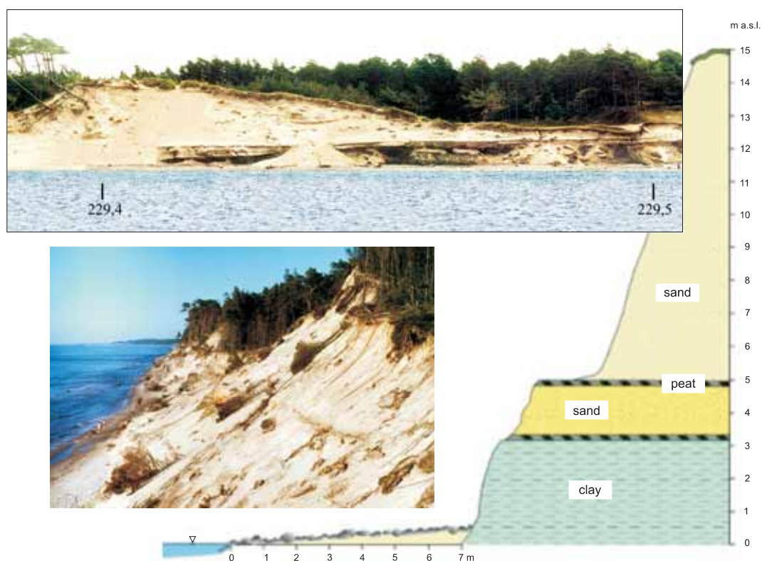
Fig. 3. Geological profile of the cliff dominated by sandy layers east from Ustka (middle Polish coast) and taluses and landslips
