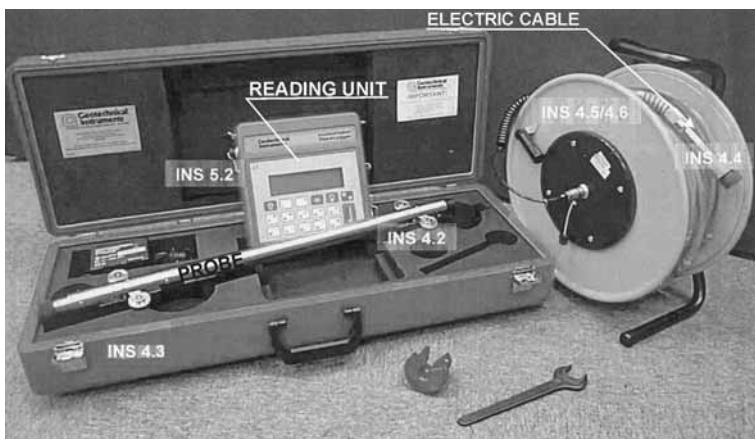
Fig. 3. Apparatus for inclinometer measurements (photograph from the User's Guide of the manufacturer "Geotechnical instruments")
