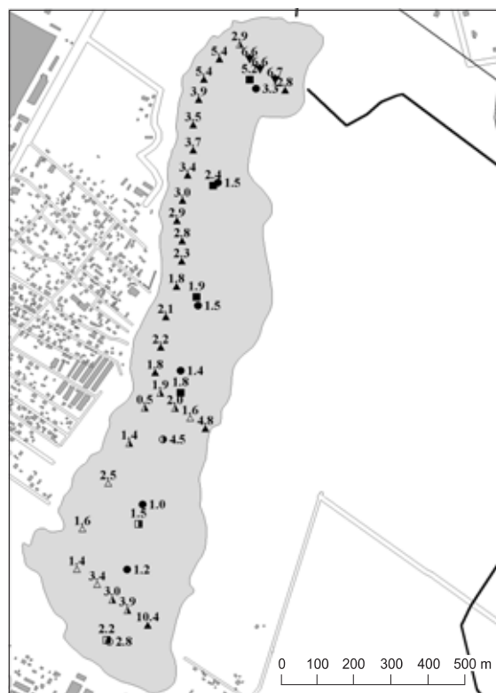
Pollution category according to Z(7) index Samples taken in: 1989 1991 2002 △ □ ○ allowable, Z(7) <10, ▲ ■ ● medium dangerous, 10 < Z(7) <30, ▲ ■ ● dangerous, 30 < Z(7) <100 ▼ ● ● extremely dangerous, Z(7) >100
