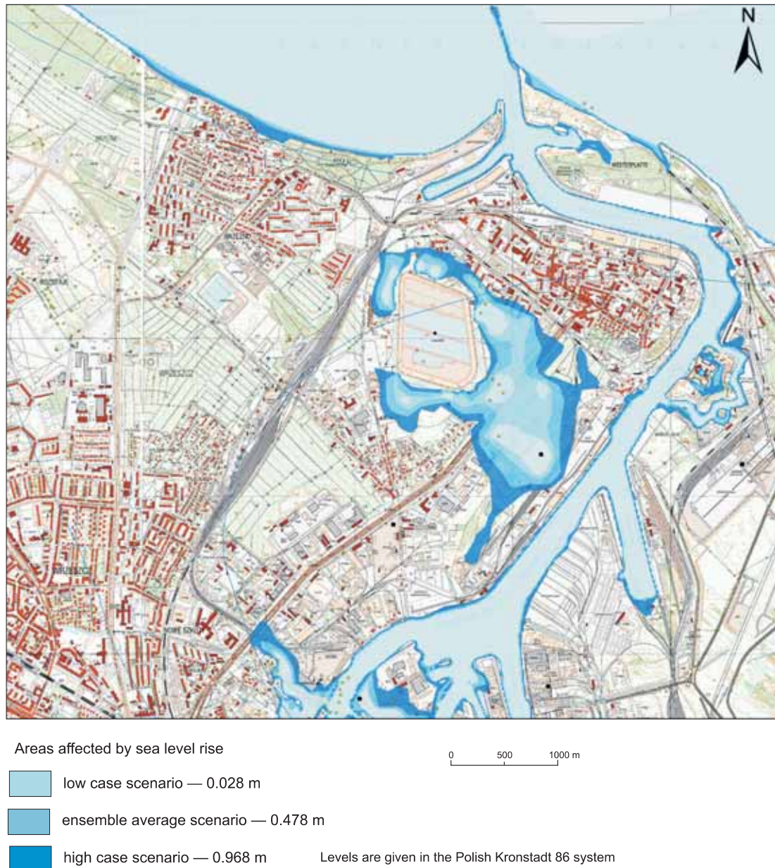
Fig. 5. Flood prone areas in the area of the Nowy Port following the SEAREG sea level rise scenarios
