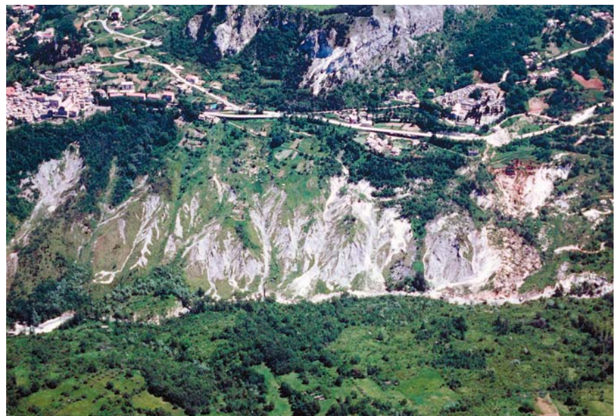
Fig. 4. Widespread, mostly shallow mass movements on May 1991 near the Caramanico's centre (left side of photo)
