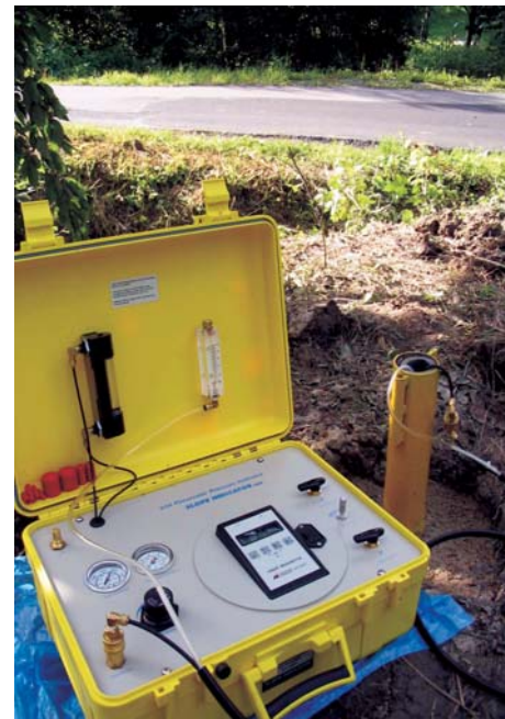
Fig. 18. Pore pressure measuring equipment
