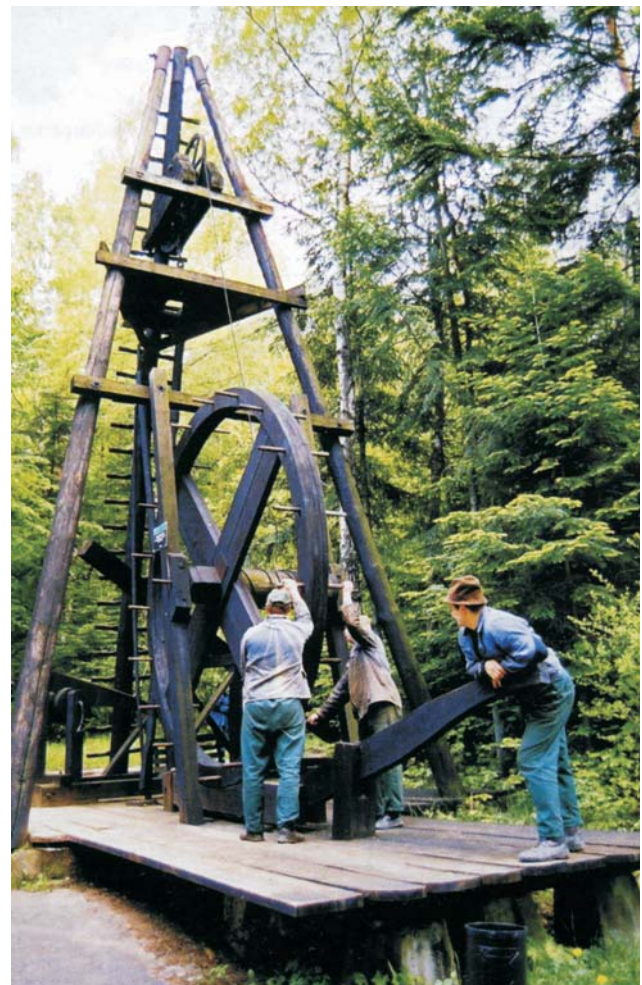
Fig. 4. Equipment for manual borehole drilling; Museum of Petroleum Industry in Bóbrka (after Garncarski et al, 2001)
