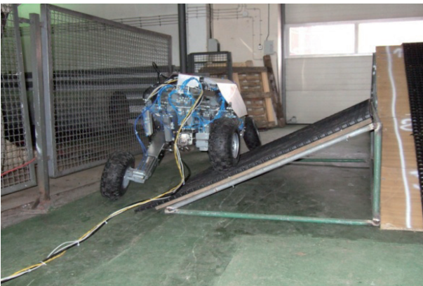
Fig. 23. Driving through a 30° side slope (rear view)
