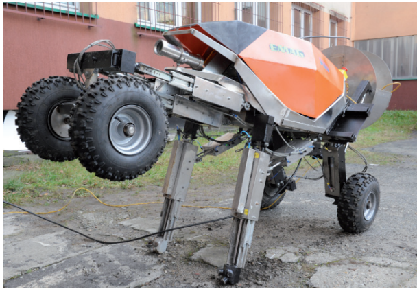
Fig. 16. Motion systems: 1 – wheel system, 2 – support system
