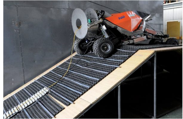
Fig. 24. Going uphill of a 30° slope
