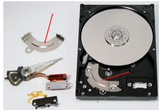
Figure 5. HDD during components disassembly – arrows pointing glued magnets
