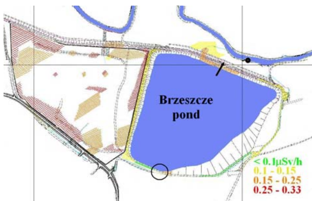
Fig. 3. Measured spatial equivalent gamma dose rates in the vicinity of the Brzeszcze sedimentation pond. As in Fig. 2 inflow pipe is indicated by circle and arrow denote outflow.
