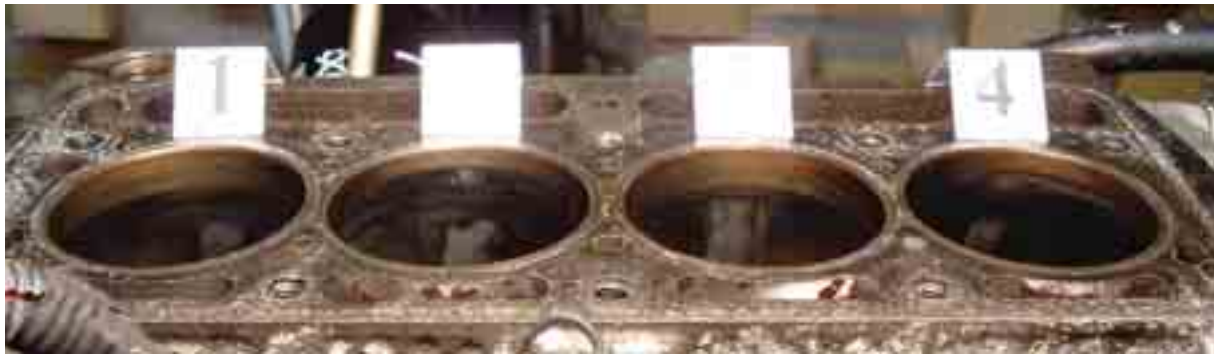
Fig. 6. View of the engine block after test, removing the pistons and removing deposits
