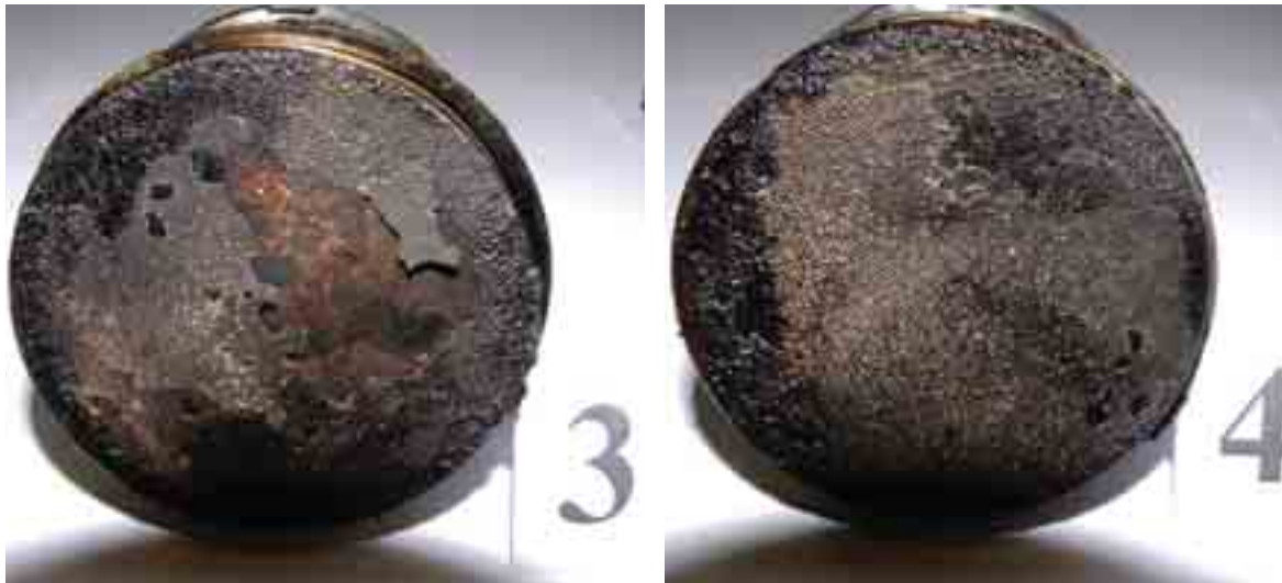
Fig. 8. View of the pistons after tests
