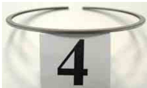
Fig. 5. View of side surface of the first ring of the cylinder No. 4
