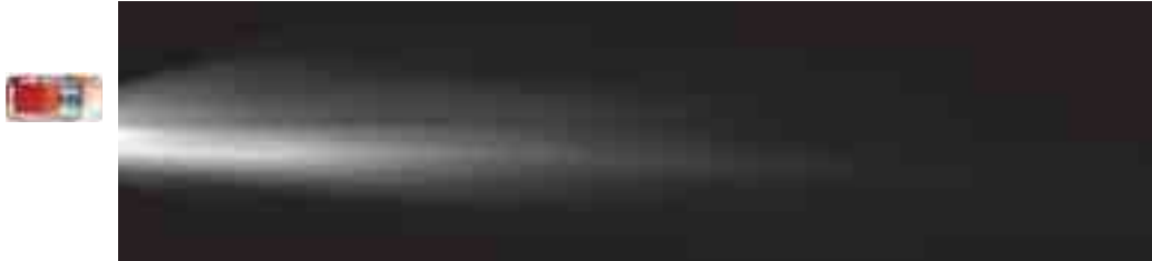
Fig. 3. Bird-eye view visualisation of vertical illumination at the road surface corresponding to object illumination on the road and their visibility
