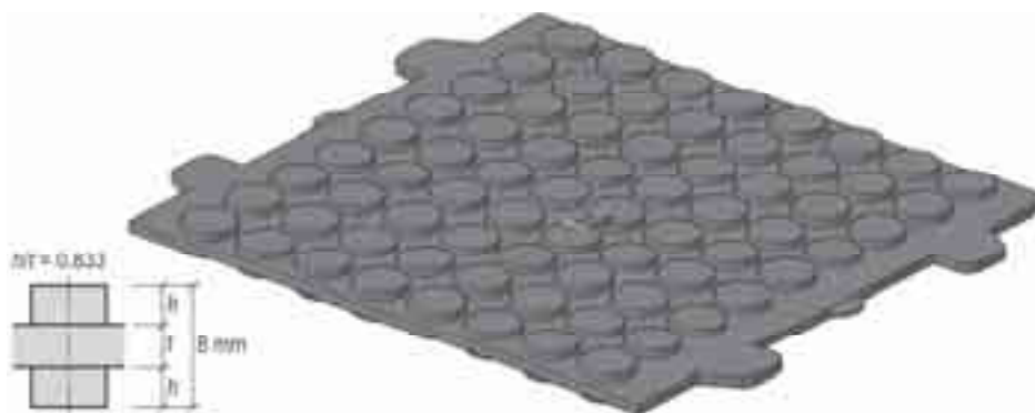
Fig. 2. CAD model of the two-sided rail pad selected for the study
