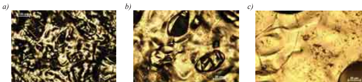
Fig. 5. MM images of 4 (three-layer system: CuZnNi / NiCuFe / CuSn) sample surface a) the scale of 100 \mu m, b) the scale of 50 \mu m, c) the scale of 20 \mu m
