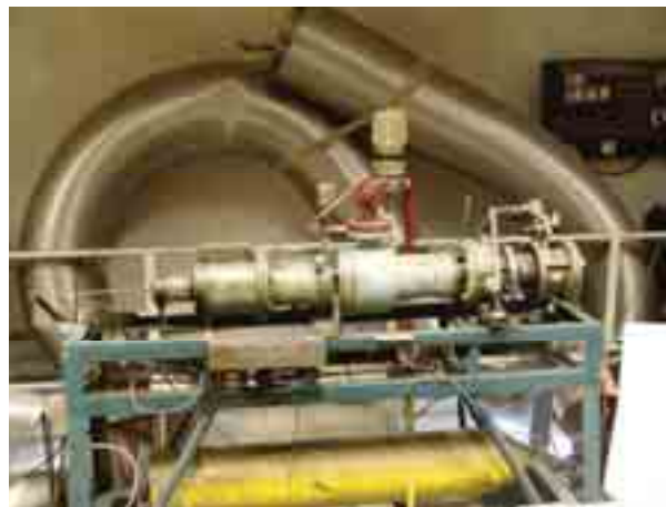
Fig.2. View of pneumatically driven RCM
