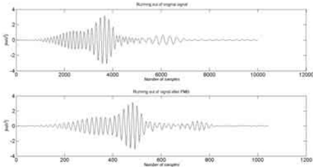
Fig. 7. Comparison of time-body vibration acceleration signal after filtering in the frequency of resonance of the unsprung masses - filling 50%: Top: primary signal, Bottom: secondary signal - after treatment with PMD
