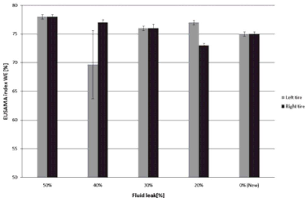
Fig. 1. EUSAMA index values as a function of fluid loss obtained for the Fiat Seicento 900 front suspension - own work based on [3]
