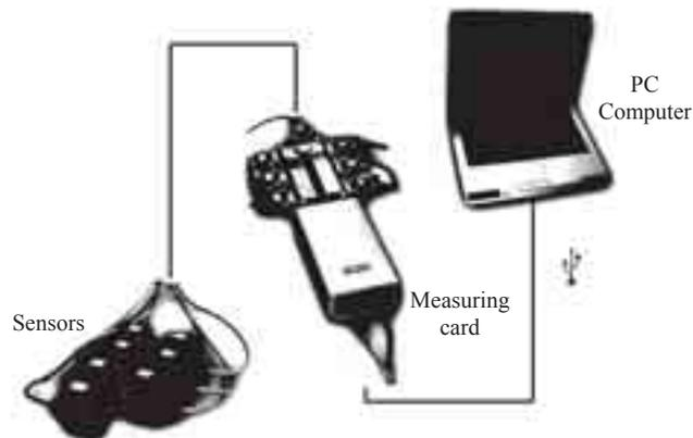
Fig. 3. The measuring vibration system [4, 5]
