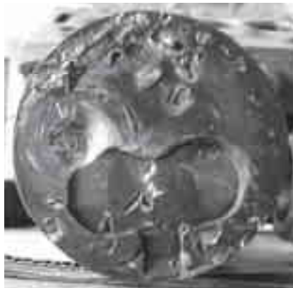
Fig. 8. Piston damage due to incorrect engine timing
