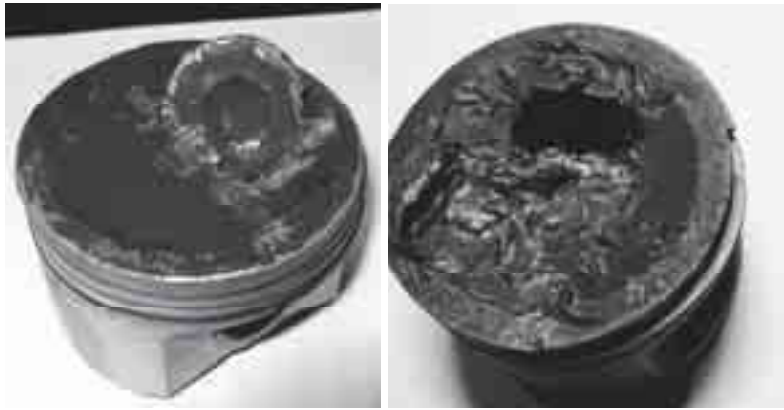
Fig. 7. Piston crown damage due to hitting against the valve
