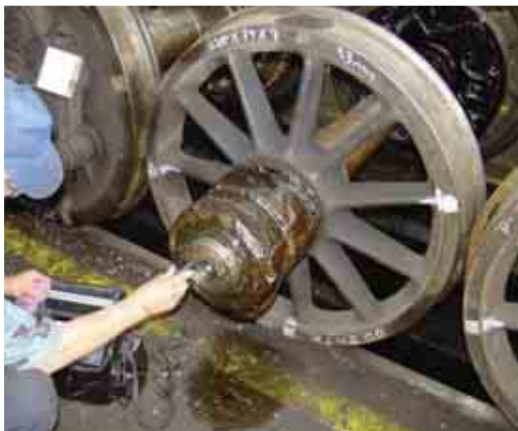
Fig. 4. Material flaw inspection of the front axle shunting locomotives SM42
