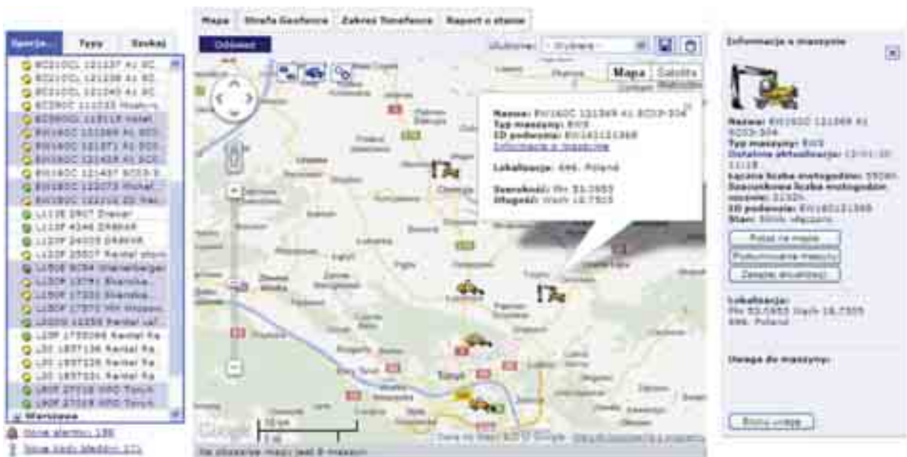
Fig. 2. Establishing the position of a selected vehicle with the use of a telematics diagnostic system
