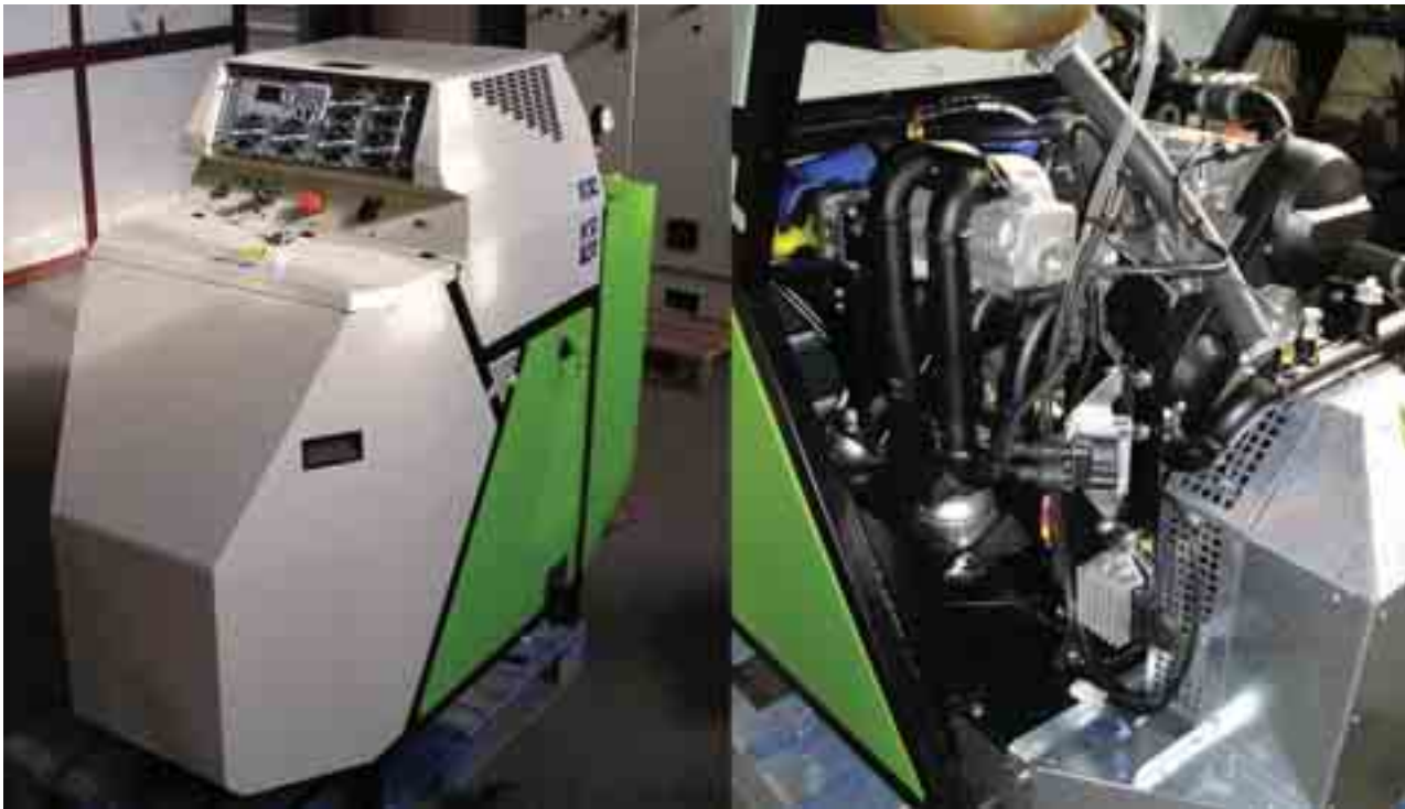
Fig. 10. Manufactured prototype of the micro-cogeneration unit (left) and an insight view of the engine with modified long intake pipes (right)
