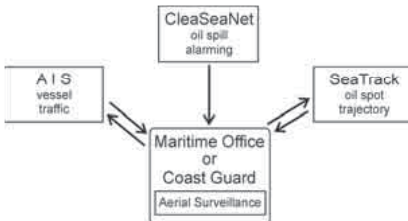
Fig. 6. The Baltic operational system for oil spill detection and source identification
