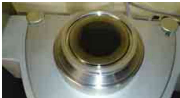
Fig. 3. Bottom plate of the rheometer, after 1319h of the oil exploitation time
