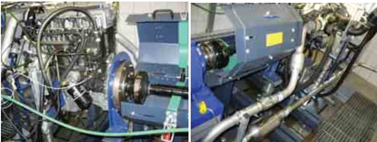
Fig.3. The ADCR engine on the test bed; The exhaust train of the ADCR engine mounted on the test bed
