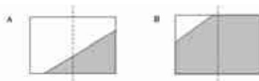
Fig. 3. Possible contact of liquid surface with tank's bottom (A) or its top (B)
