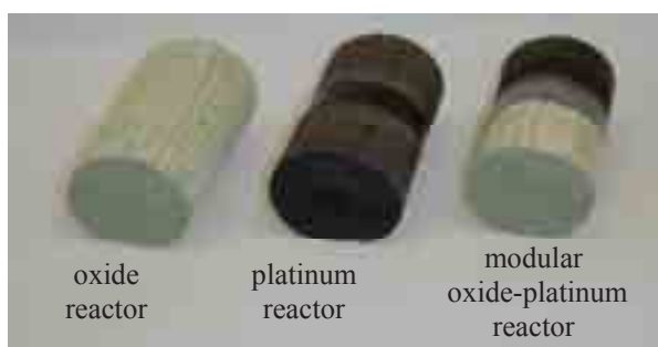
Fig. 1. A picture of three reduction reactor models tested used in the NH 3 -SCR system
