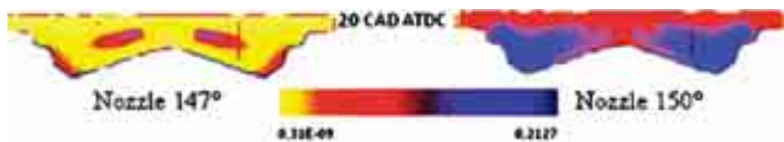
Fig. 8. Air-fuel mixing comparison between the 147°(left side) and 150° (right side) nozzles. (Operative condition: SOI=20 cad ATDC)
