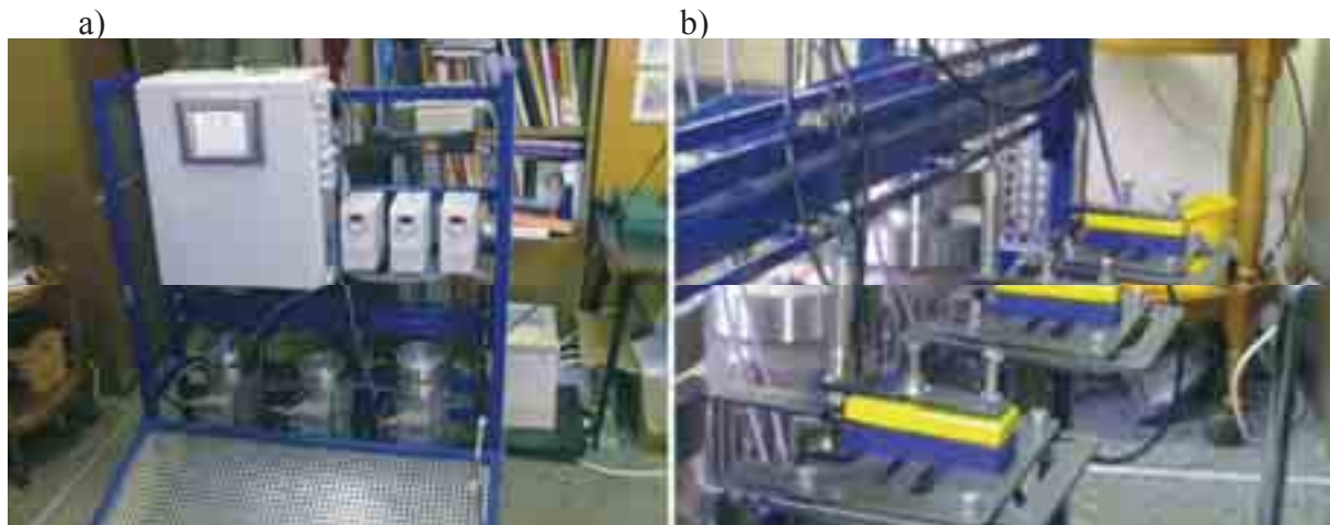
Fig. 4. NMZ-1 Neodymium Fatigue Testing Machine, a) – general view; b) view of clamp section and measurement sensors
