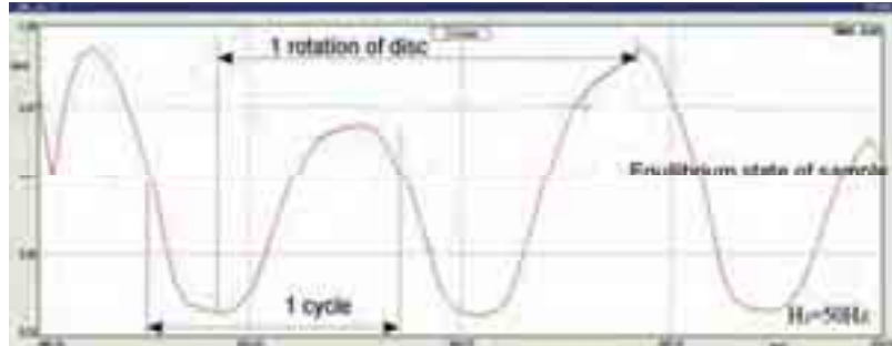
Fig. 9. Displacement range of a material point in the sample at rotational frequency of 50 Hz, excitation – double disc
