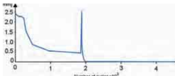
Fig. 14. Changes in the amplitude of sample displacement during test cycles – the sample was damaged
