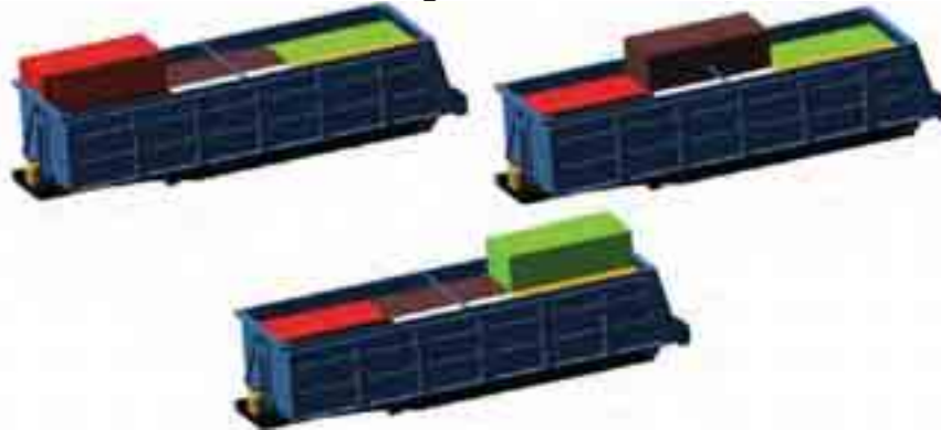
Fig. 1. Non-uniform cargo distribution. Simulations only for one-side changes, because of the construction symmetry
