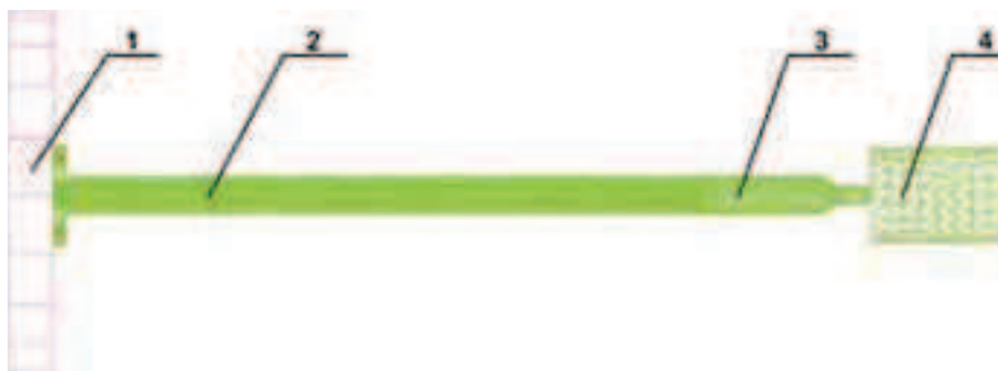
Fig. 7. Numerical model of lance without frictional damper: 1) stationary cast iron block, 2) lance, 3) transition element (end), 4) equivalent mass
