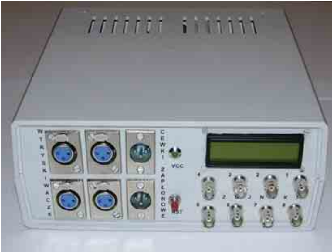
Fig. 2. Controller’s front panel for batched injection
