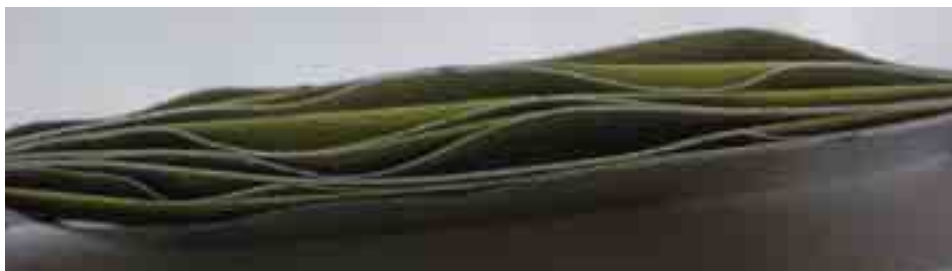
Fig. 14. Delaminated specimen of laminar composite
