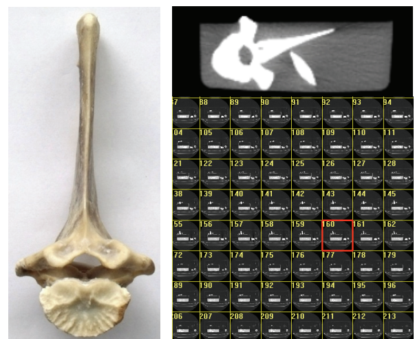
Fig. 6. View of a pig spinal vertebra and image of a pig spine measurement on tomography
