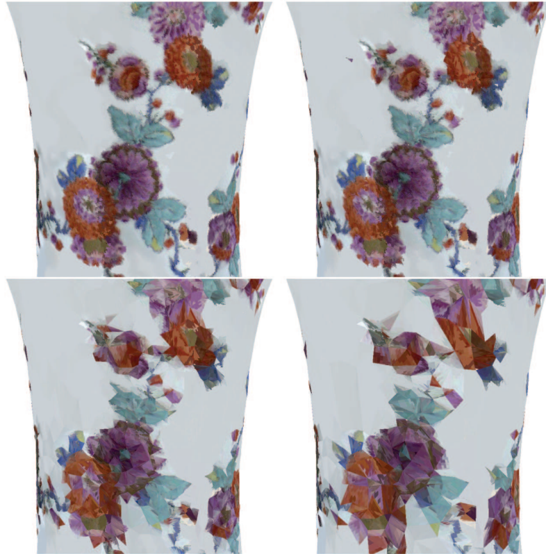
Fig. 2. Comparison of texture representation quality. Original (top left), reduction ratio = 0.5 (top right), reduction ratio = 0.1 (bottom left) and reduction ratio = 0.05 (bottom right)
