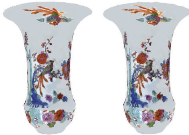
Fig. 1. Textured mesh waza.obj (134227 faces). Original (left) and decimated (right)
