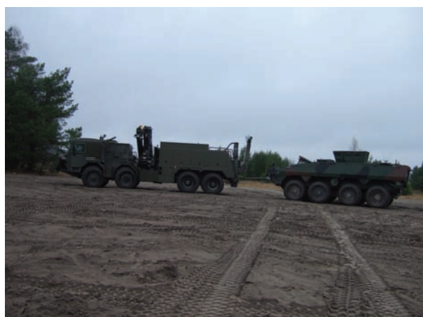
Fig. 8. View of the vehicle while performing a towing test of a damaged AMV Rosomak vehicle in its base version with a turntable using the tow-rod
