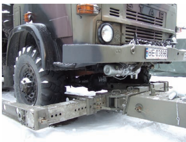
Fig. 15. View of the way to join hydraulic hoisting and towing device to Star 266 vehicle by using tow-hitches for wheels slipped-on a cross bar (traverse) and the tow-hitches for (opposite) wheels before a towing test is performed
