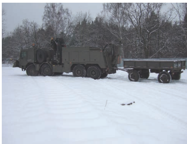
Fig. 12. View of the vehicle while performing a towing test of a D-46-type of damaged biaxial trailer, using a towing hook
