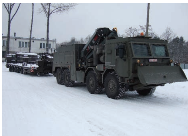
Fig. 13. View of the vehicle while performing a towing test of a damaged N-60W-type of flatbed, using the lifting and towing device by the front of the damaged vehicle
