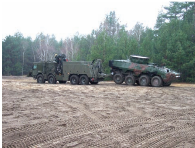
Fig. 11. View of the vehicle while performing a towing test of a damaged AMV Rosomak vehicle in its base version with a turntable using the lifting and towing device by the rear of the damaged vehicle
