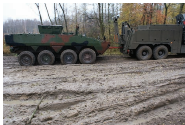
Fig. 9. View of the vehicle while performing a towing test of a damaged AMV Rosomak vehicle in its base version with a turntable using the tow triangle
