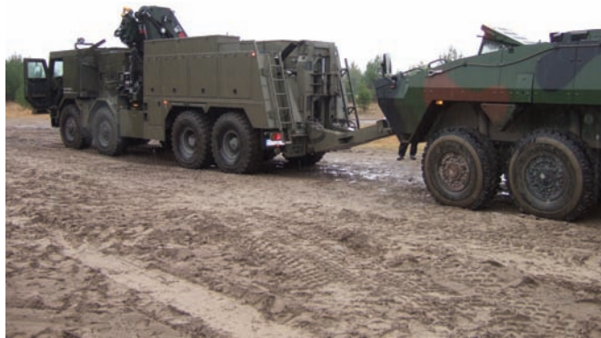
Fig. 10. View of the vehicle while performing a towing test of a damaged AMV Rosomak vehicle in its base version with a turntable using the lifting and towing device by the front of the damaged vehicle
