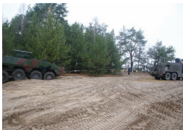
Fig. 14. View of the vehicle while performing an evacuation test of the bogged down damaged AMV Rosomak vehicle in its base version with a turntable using the main winch
