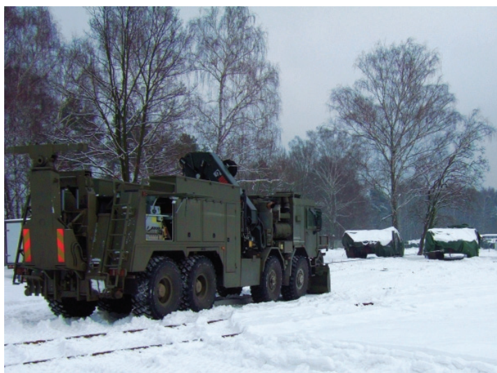
Fig. 6. View of the vehicle while performing the test to measure traction force of the winch for self-evacuation
