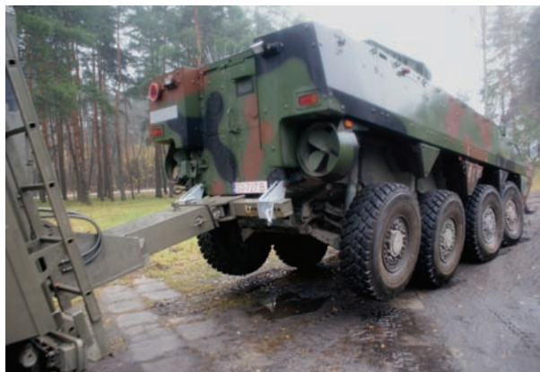
Fig. 7. View of the hydraulic hoisting and towing device in the vehicle while performing the load position stability test (protection against self-lowering when loaded with a damaged AMV Rosomak vehicle in its base version with a turntable)
