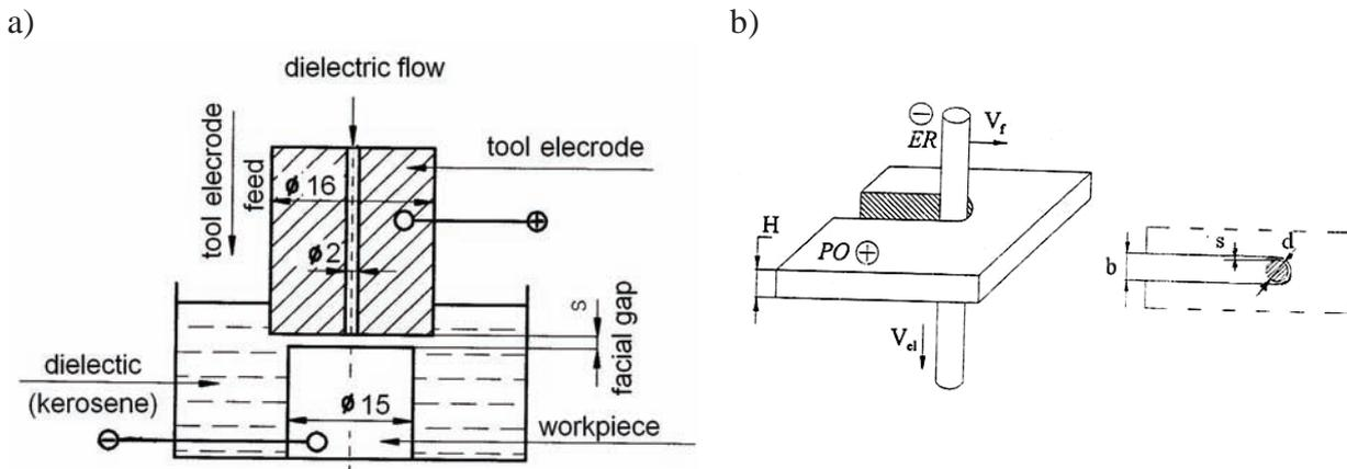
Fig. 4. Diagram of different electrical discharge machining methods applied in the studies: a) sinker (EDM), b) wire erosion (WEDM)
