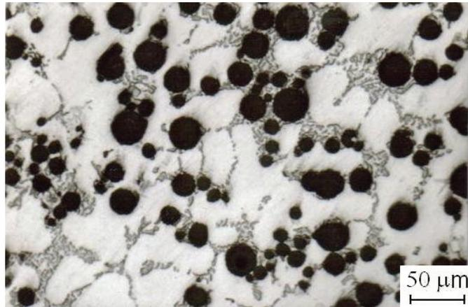
Fig. 5. Microstructure of composite material AlSi7Mg+20% Al<sub>2</sub>O<sub>3</sub>
