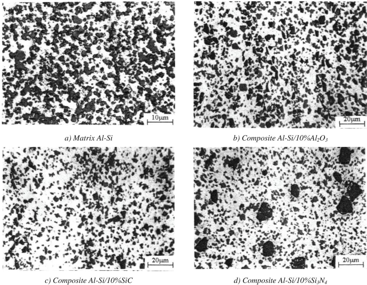
Fig. 6. Metallographic microsections of: (a) matrix (ASCM) –K0; (b) composite with 10%  $Al_2O_3$  –KA3; (c) composite with 10%SiC– KS3; (d) composite with 10% $Si_3N_4$ – KN3 [1]
