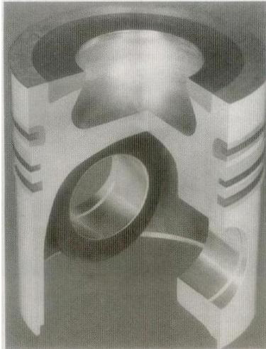
*Fig. 2. First piston of composite materials from TOYOTA [11]*
