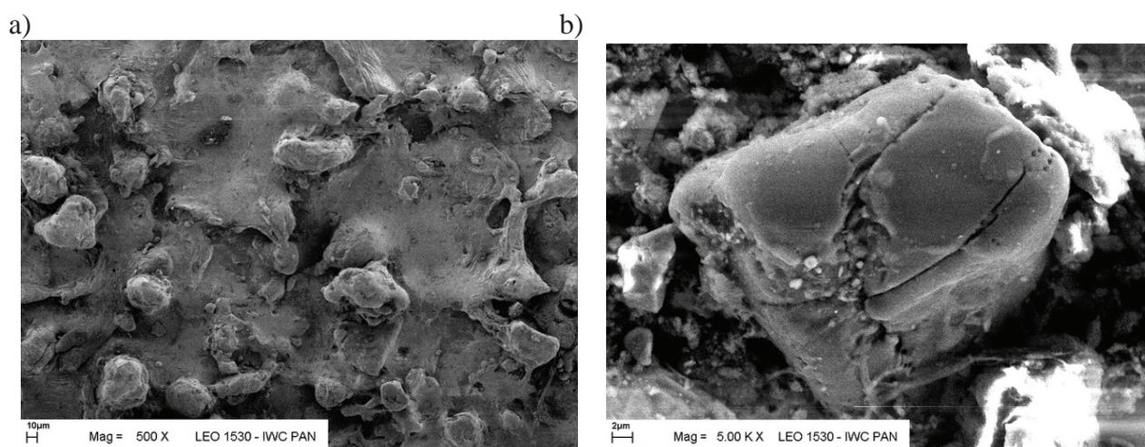
Fig. 11 Surface SEM after EDM of Al. + Al<sub>2</sub>O<sub>3</sub> composite with granularity 53 μm a) and a single adhered to the surface b) [8]
