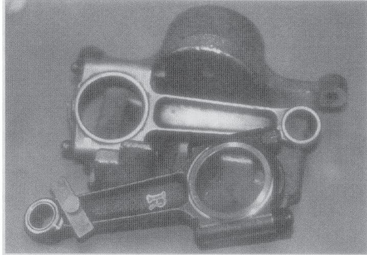
*Fig. 3. Connecting rods of Al. composite material reinforced with Al<sub>2</sub>O<sub>3</sub> continuous fibre for a Ferrari car. Steel connecting rod weight 485 g, composite material connecting rod [11]*
