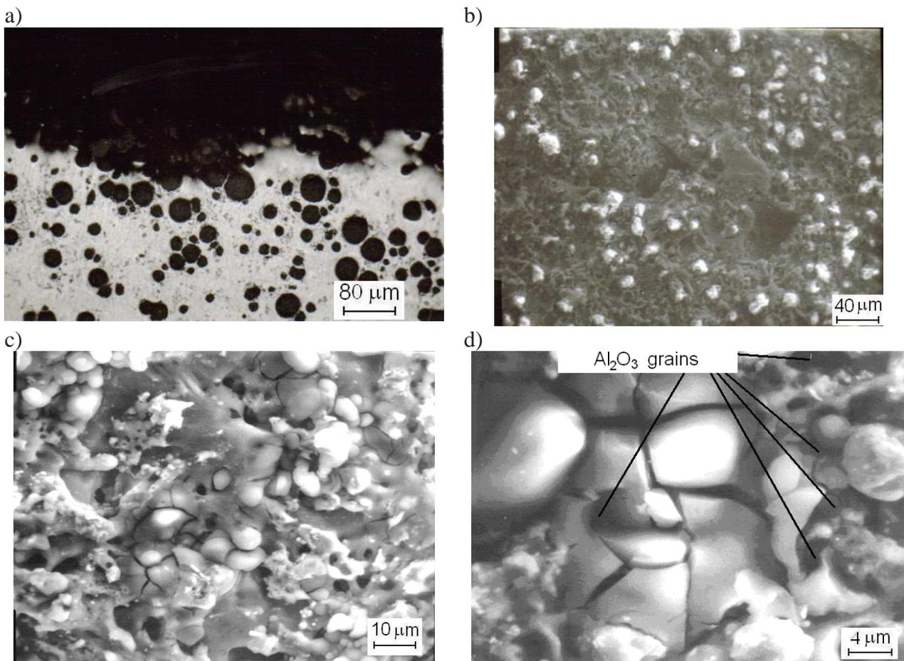
Fig. 9. surface SEM after electrical discharge machining of composite Al. + 20% Al<sub>2</sub>O<sub>3</sub>: a) after EDM ( $I = 16A$ ,  $t_i = 500 \mu s$ ,  $t_o = 112 \mu s$ ); b, c and d) after WEDM ( $U = -120V$ ,  $I = 16A$ ,  $t_i = 1.2 \mu s$ ,  $t_o = 5.8 \mu s$ ) [8]
