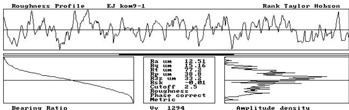
Fig. 10. Examples of post-EDM surface roughness profilograms: (a) for matrix material; (b) for composite material with 10% (by volume) of  $\text{Si}_3\text{N}_4$  reinforcement
