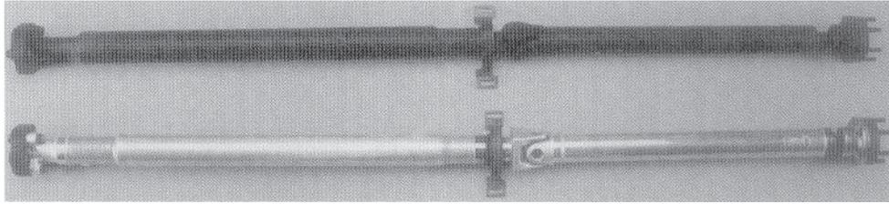
*Fig. 1. Driveshaft of Al. alloy for plastic working, reinforced with SiC particles [11]*
