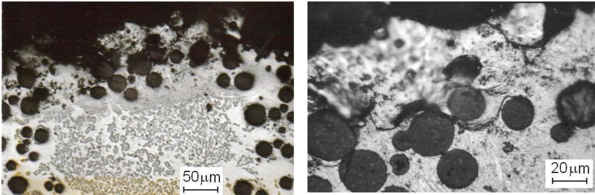
Fig. 8. Metallographic structure after EDM of composite Al+20% Al<sub>2</sub>O<sub>3</sub> a and b) ( $I=16A$ ,  $t_i=1000\mu s$ ,  $t_o=250\mu s$ ) [8]
