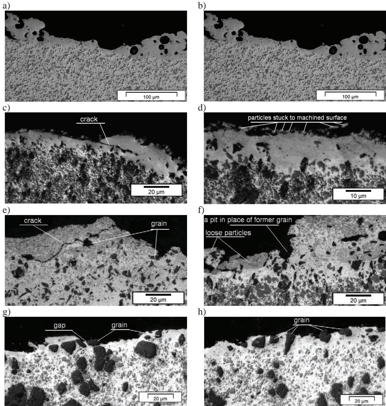
*Fig. 7. SL microstructure after EDM: a and b) matrix KO ( $I = 16 \text{ A}$ ,  $t_i = 500 \mu\text{s}$ ,  $\sigma = 0.6$ ); c and d) composite KA3 ( $I = 16 \text{ A}$ ,  $t_i = 500 \mu\text{s}$ ,  $\sigma = 0.6$ ); e and f) composite KS3 ( $I = 16 \text{ A}$ ,  $t_i = 500 \mu\text{s}$ ,  $\sigma = 0.6$ ); g and h) composite KN3 ( $I=10\text{A}$ ,  $t_i = 266 \mu\text{s}$ ,  $\sigma = 0.6$ ) [8]*
