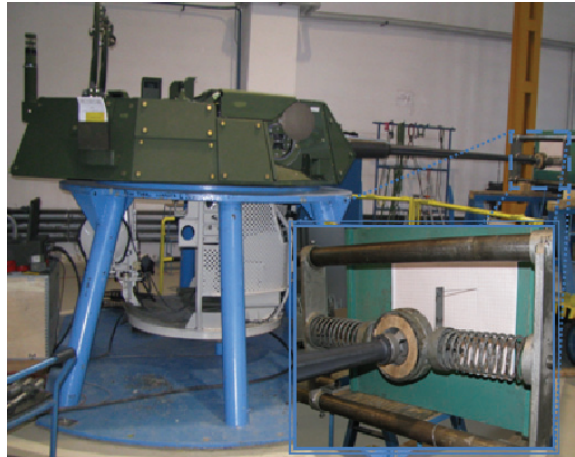
Fig. 4. Measurement stand with equipment to measure inertia moment of the turret
