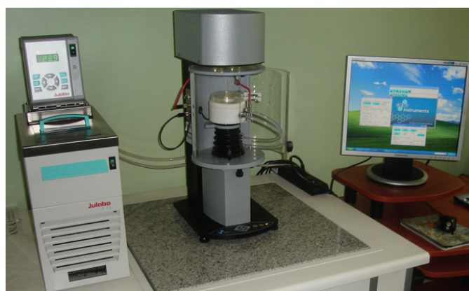
Fig. 2. Testing station for the measurement of density, surface tension and wetting angle
