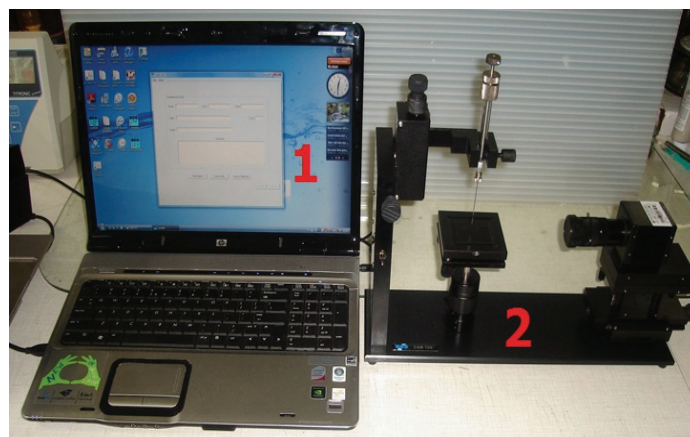
Fig. 5. Test stand for measurement of static wetting angle: 1 – notebook for test control with appropriate software installed; 2 – KSV CAM 100 apparatus
