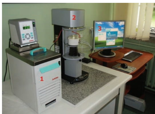
Fig. 3. Test equipment for measurements of density, surface tension and dynamic wetting angle: 1 – JULABO F-12 thermostatic bath; 2 – KSV Sigma 701 tensiometer; 3 – personal computer for test control
