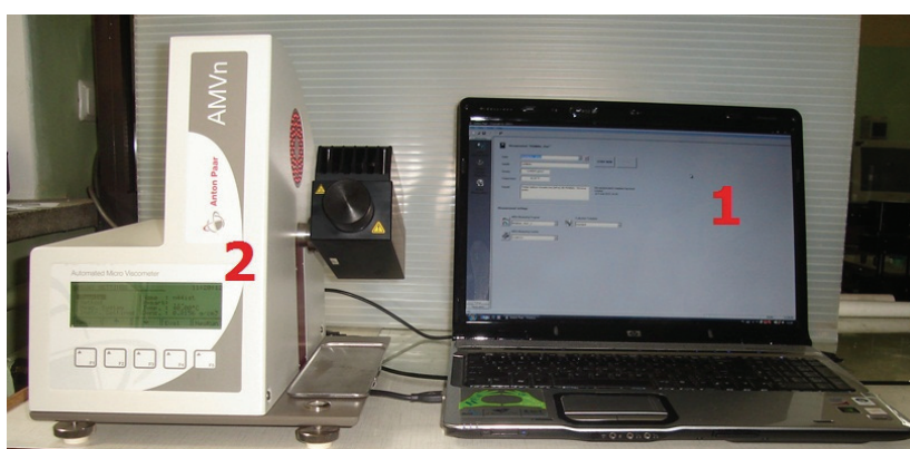
Fig. 6. Test stand for measurements of absolute viscosity: 1 – notebook for test control with appropriate software installed; 2 – AMVn viscometer
