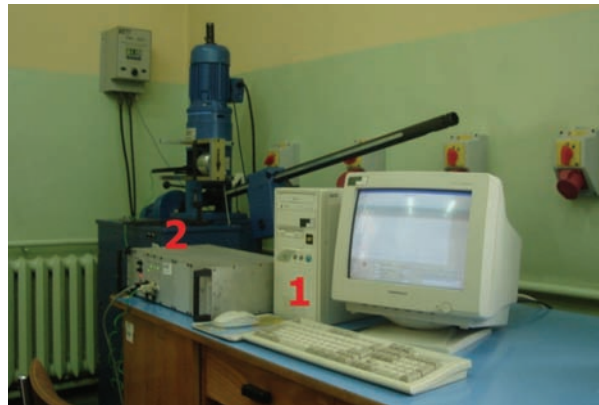
Fig. 7. Test stand for measurements of lubricity properties: 1 — personal computer for test control with appropriate software installed; 2 — T-02 four-ball apparatus with a digital amplifier and a set of transducers
