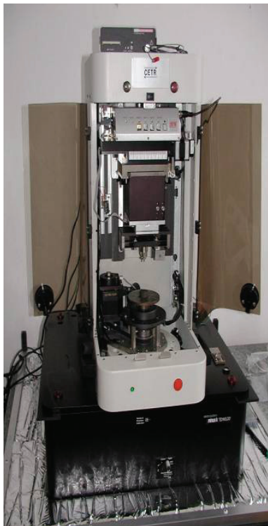
Fig. 11. UNMT research set (Universal Nano & Micro Tester), made by CETR (USA), for characterizing mechanical and tribological properties of surfaces
