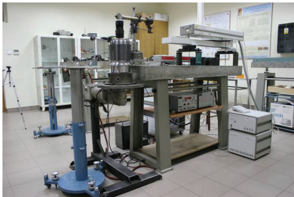
Fig. 12. General view of the stand for the laser spreading of oil microcontainers
