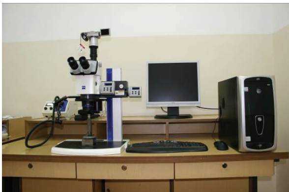
Fig. 14. Laboratory observation and archiving set for microscopic images consisting of: Discovery stereoscopic microscope, Canon camera, workstation PC
