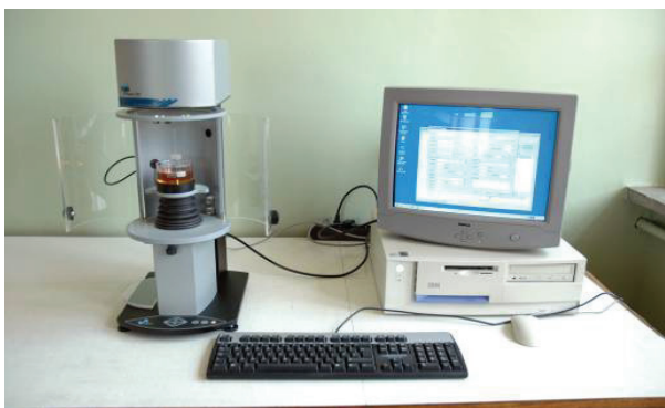
Fig. 9. KSV701 tensiometer for evaluation of the surface-energy properties of liquid lubricants
