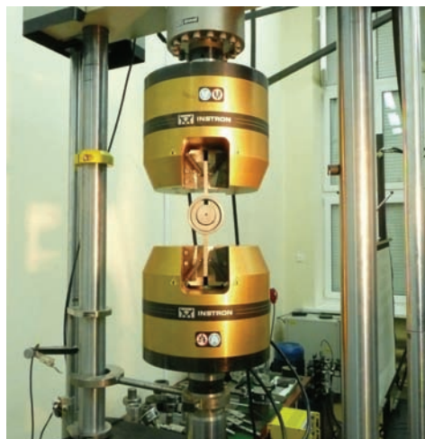
Fig. 10. The tensile strength tests of prototype coupler
